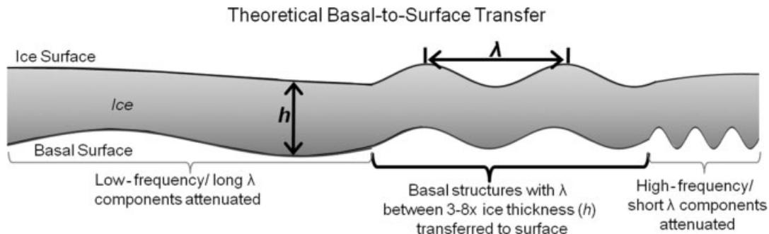
Figure 2. Schematic of basal to surface transfer as a function of ice thickness, where ( $h$ ) is ice thickness and ( $\lambda$ ) indicates surface and basal wavelength (not drawn to scale). Basal wavelength ( $\lambda$ ) components between three and eight times the ice thickness ( $h$ ) are most readily transferred through the ice whereas wavelengths longer and shorter than this 3–8 $\times$  window are strongly attenuated
