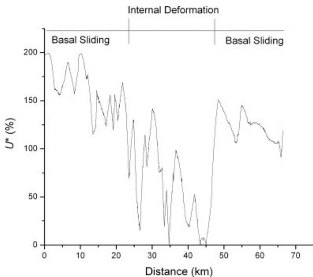
Figure 7. Relative impact of basal sliding ( $u_b$ ) to internal deformation ( $u_d$ ) on ice sheet velocity along the study transect through calculation of  $U^*$  (percent difference) between measured surface velocity ( $u$ ) and an estimate of  $u_d$  based on the depth-average velocity. High values in  $U^*$  indicate the relative importance of basal sliding to surface velocity over internal deformation
